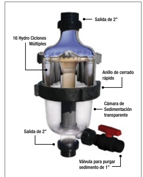
Partes del Pre-filtro Multi Cyclone
